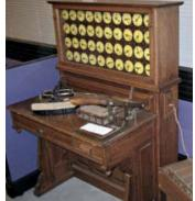
The machine was proof of his concept that data could be encoded by holes punched in a card and thereby counted and sorted electronically. It was successful, and Hollerith went on to found the Tabulating Machine Company, which later merged to become a company called IBM.
